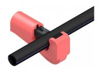
Insert the components on the pipe according to sequence that follows: nut, cut olive (external surface marks have to be directed forward the nut and not forward the fitting), compression ring and gasket (and at the end the sleeve, where expected).
